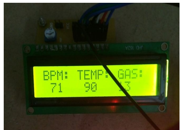
Fig : The BPM, temperature and gas values shown in LCD display.
