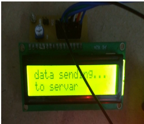
Fig : Data is uploading in server shown in LCD display.
