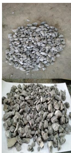
(a) virgin aggregate (b) broken concrete
