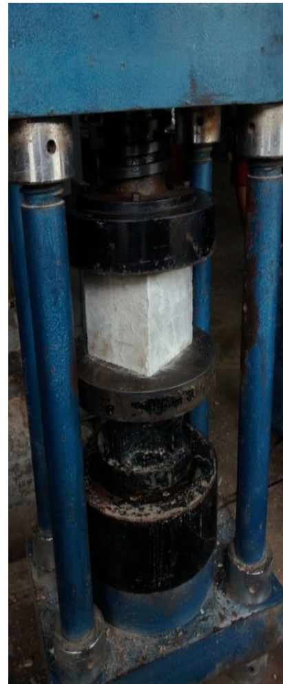
Fig. 3.3 Testing of cubes for compressive strength
