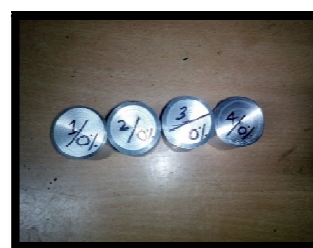
Fig 2. Prepared Specimens of Al 6063 + 0wt% of TiC
