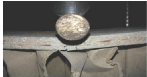
Figure 3: Bending of cement fiber board under point load
