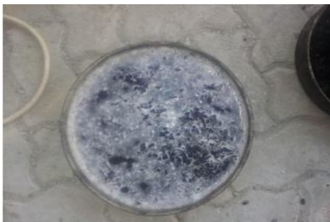
Figure 4.3 NaOH treatment on rubber tyres
