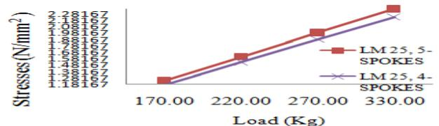
Stress Comparison between 5-Spokes and 4-Spokes alloy wheel of Aluminum Alloy (LM 25).
