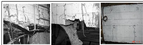
Figure 2 Failure pattern of FRP Strengthened RC Slabs
