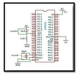
The 89S52 is a low power, high performance CMOS 8 bit microcomputer with 8k bytes of flash programmable and erasable read only memory (PEROM).The device is manufactured using Atmel's high density nonvolatile memory technology and it is compatible with the industry standard 89S51 and 89S52 instruction set and pin out.
