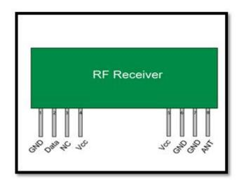
It uses ASK (Amplitude Shift Keying) conventional heterodyne receiver IC for remote wireless applications.
