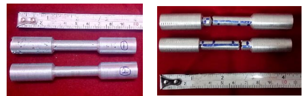
(a) Before Test (b) After Test figure 2 Tensile Test specimens
