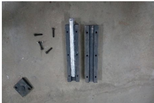
Fig 2: Obtained composite from mould
