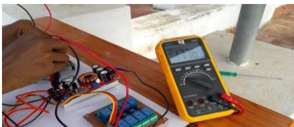
Figure 7.1 PV panel output voltage
