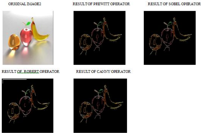
Fig2: Performance of Prewitt, Sobel, Robert, Canny edge detectors on Image2
