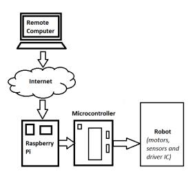
About Raspberry Pi: It is nothing but a debit card sized small CPU. Its similar to our conventional desktop PCs. It has on board ARM processor, Graphic processor, memory, USB slots, Ethernet, Wi-Fi, Bluetooth, HDMI output, audio jack, etc.
