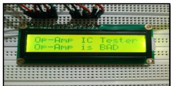
Fig. 8 Testing of Non-working IC-741
