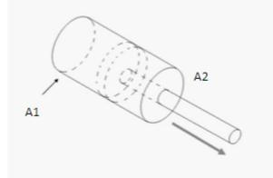
A1-area of outstroke A2-area of in stroke  $A1 = \pi r^2$  =r=D/2=32/2=16mmA1=3.14\*16\*16 A1=804.25mm squ......(1)  $A2 = \pi r^2$  A2 = r=D/2=12/2=6mmFrom paper of GRANTA piston dia is for 32 bore = 12 mm A2 = 3.14\*6\*6 A2 = 113.04mmsqu.....(2)
