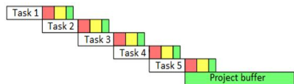
Figure 1 Buffer placed in the end of a chain protects her from delays.[2]
