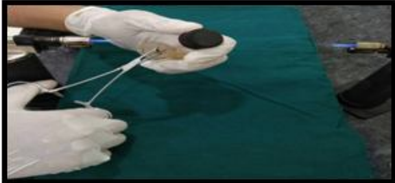
Plate--5: Plunging of Implant/Abutment unit in the bacterial suspension
