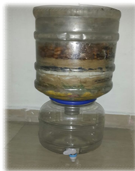
Figure 1. Model of Bio Mechanical Filter
