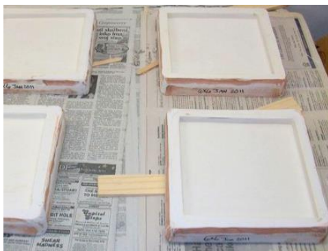
Fig.1: Mould for casting of tiles
