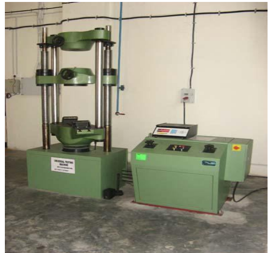
Figure : Universal testing machine used to determine the tensile strength of the welded pipe specimen
