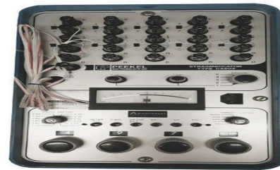
Fig. The tool used to measure the strain generated from the Wheatstone bridge to measure resistance in a strain gauge. Following is an example of how the stress is calculated from measurements:
