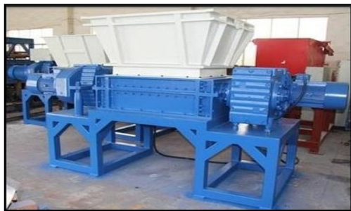
Fig.3: - Plastic shredding machine
