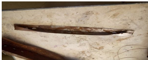
Fig 10 Failures due to block shear of single equal angle specimen with Lip 70x70x2
