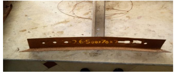
Fig 5 Failures due to tearing in bolts of single angle specimen 70x70x2
