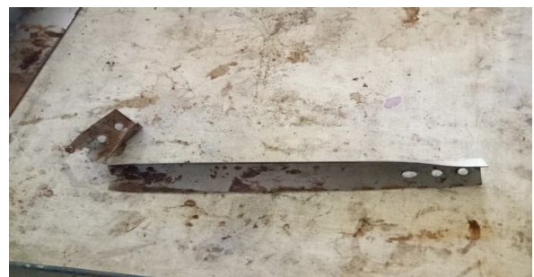
Fig 8 Failures due to block shear of single equal angle specimen 50x50x2
