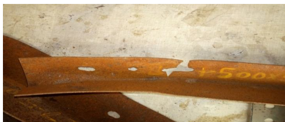
Fig 12 Failures due to net section of single angle specimen 50x50x2
