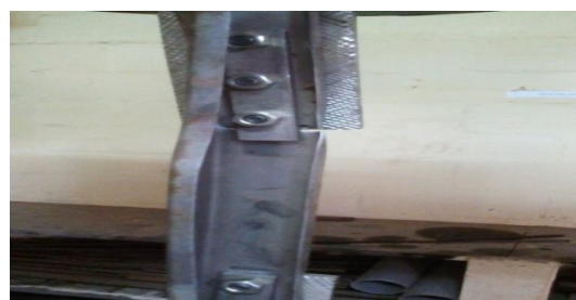
Fig 2 Failure due to local bending of single angle with Lip
