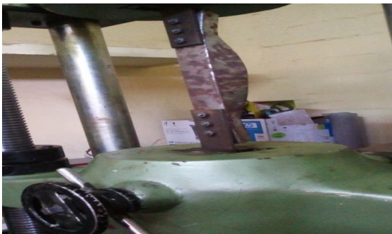
Fig 4 Failures due to local buckling of single angle specimen 70x70x2
