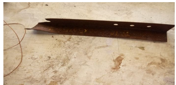
Fig 7 Failures due to block shear of single equal angle specimen 50x50x2
