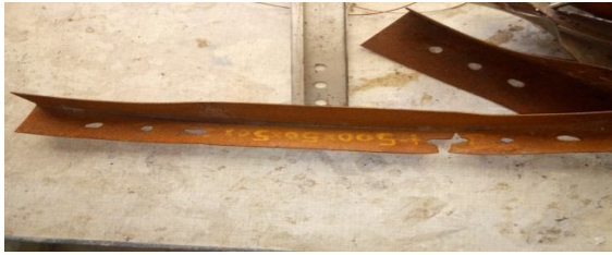
Fig 3 Failure due to local bending
