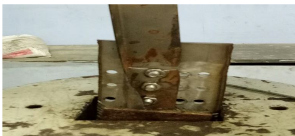
Fig 11 Failures due to net section of single un equal angle specimen 70x35x2
