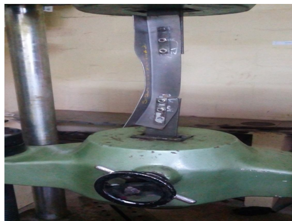
Fig 1 Failure due to global bending of single plain angle specimen
