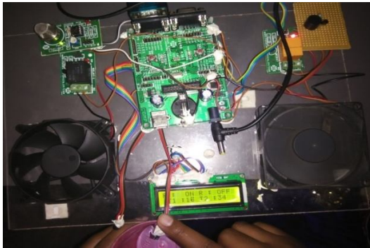
Fig.Sensor Reading Indication of Low Temperature
