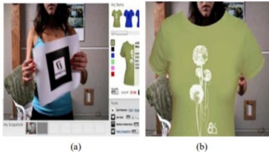
Figure 8. (a) Application search for the marker; (b) Marker replacement with a virtual object [17].
