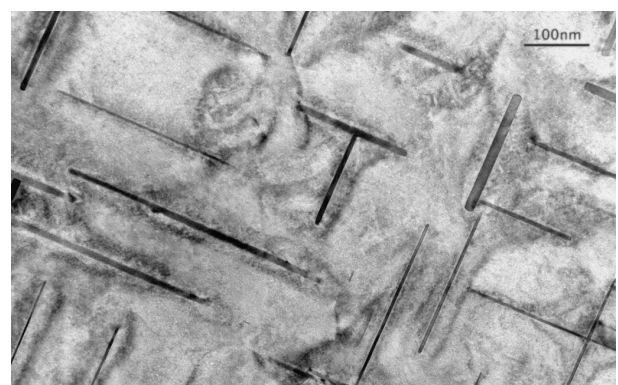
Figure 1.5 Aluminum copper (4 at% Cu) alloy showing copper precipitation within the aluminum matrix.
