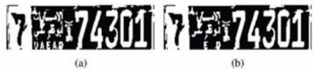
Fig. 17: (a) Binarized Image using adaptive thresholding (b) Image after applying morphological operations
