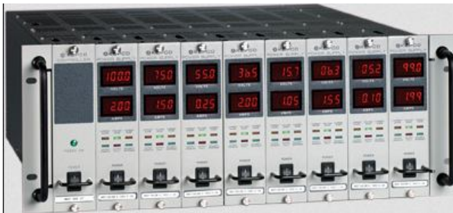
Fig.4) Example of Switch Mode Power Supply Rack [7]
