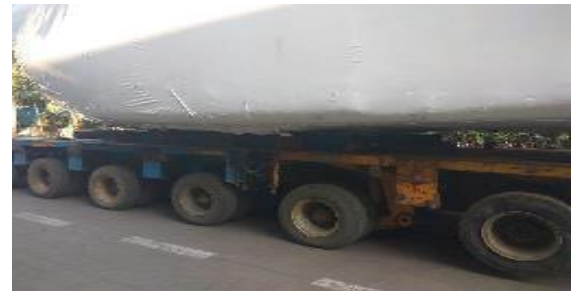
Fig.19. Nacelle road transportation
