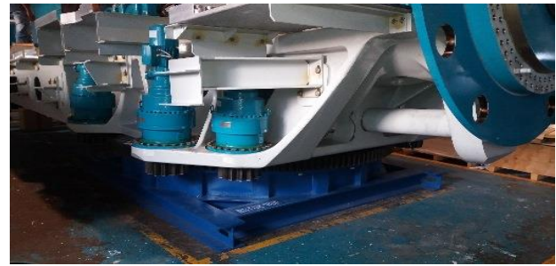
Fig.18. Nacelle carrier assembled in nacelle
