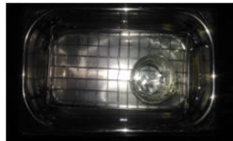
Fig 4: Ultrasonic setup to clean the substrate
