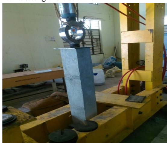
Fig-3: Column Test Setup
