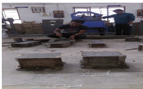
Casting of Cubes and Beams
