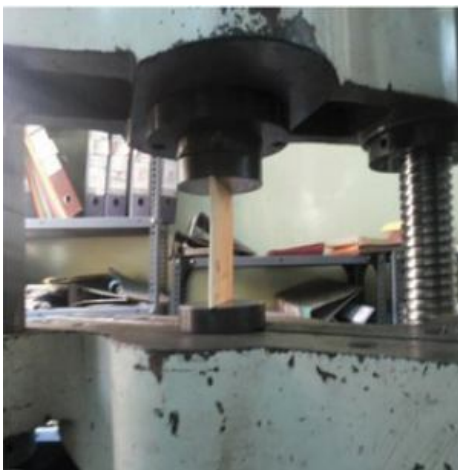
Figure 3. Specimen before buckling
