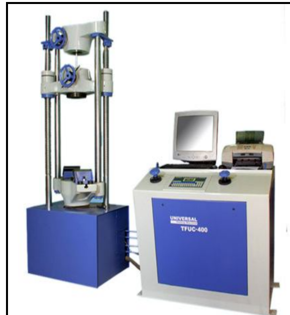
Fig 4.4:- Universal Testing Machine
