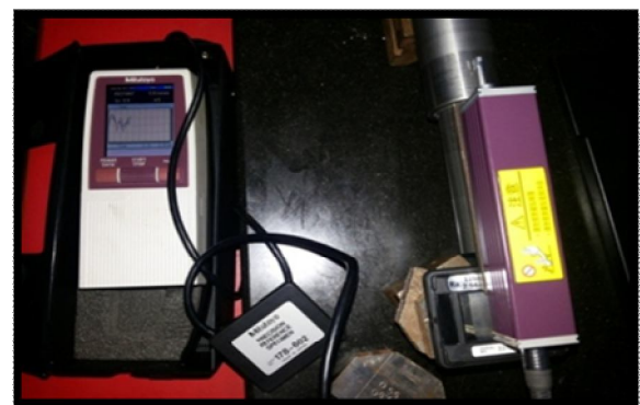
Figure 3. Mitutoyo surface Roughness Tester SJ-210
