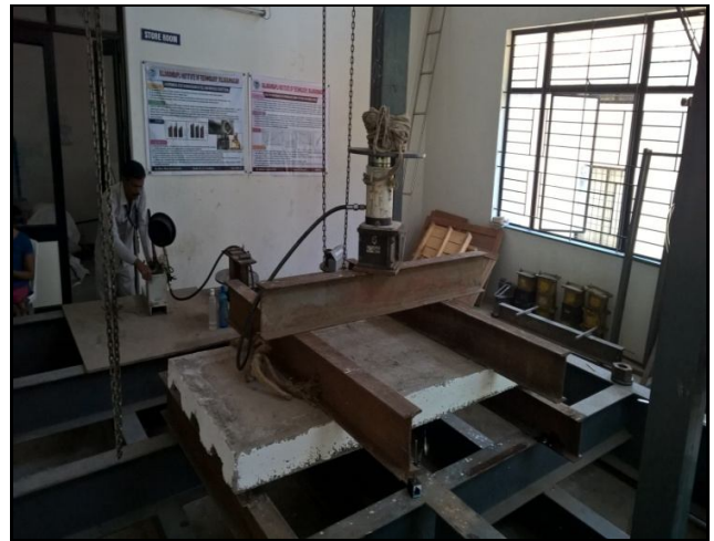
Figure 1 - Loading Setup for Slab Testing
