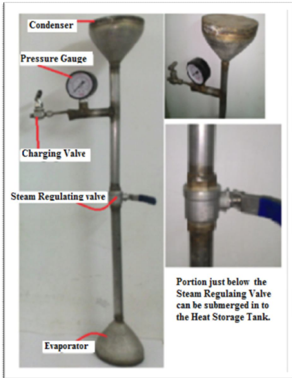
Fig. 2: Boiler Based Heat Pipe
