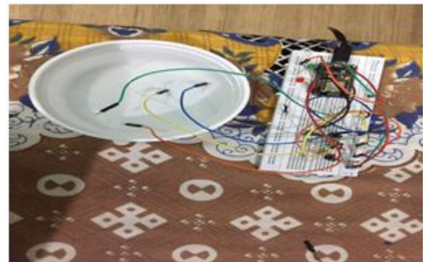
Fig. 12. water level indicator circuit
