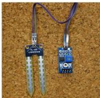
Fig. 2. Soil Moisture Sensor
