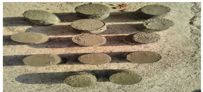
Fig 3. Filling of empty Plastic Bottles with mortar using Demolished Material as coarse aggregate.
