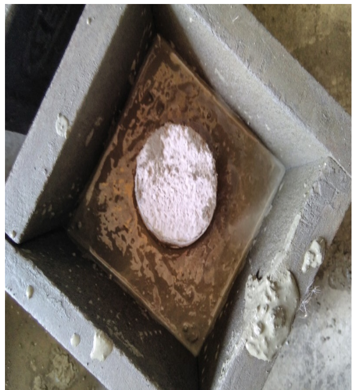
Fig 4. Placing of Plastic Bottle filled with Demolished Material into M25 Cube.
