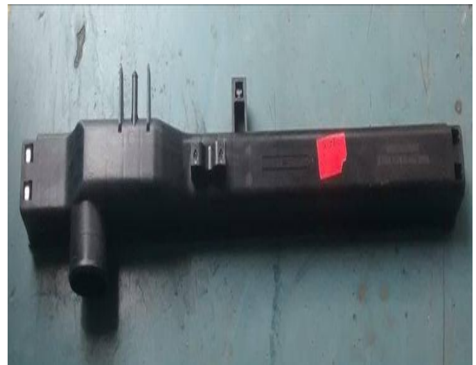
Figure 2 b. Radiator Upper tank top view
