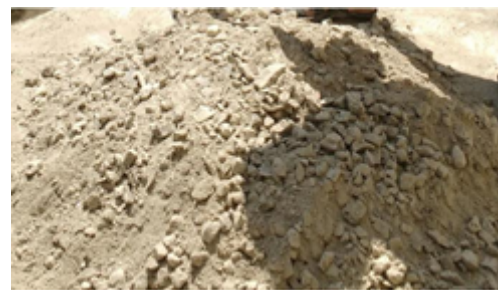
Figure 1. Dry mixture of Geopolymer concrete
