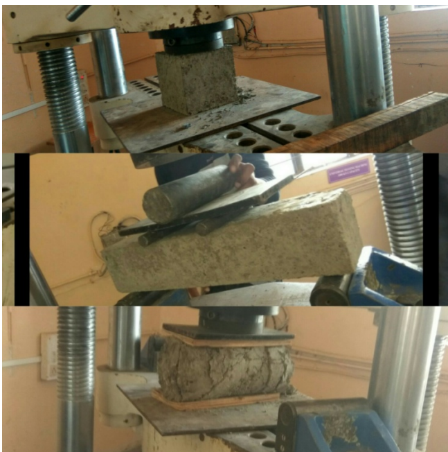
Figure 5. Compressive, flexural, split tensile testing setup.
