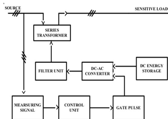
Figure 3 Function blocks of designed DVR
