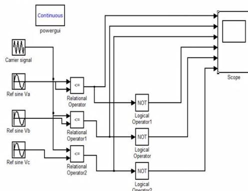
Figure 23: Generation of Gate Pulse
