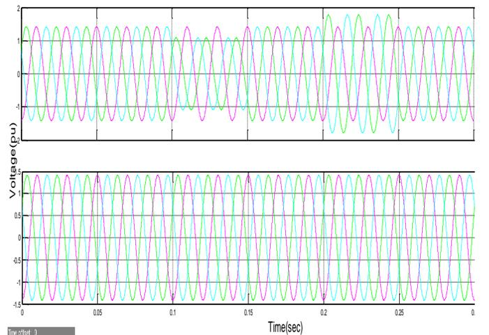
Figure 17: Simulation result of supply voltage and reference voltage in the event of sag and swell in one phase
