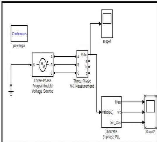
Figure 7: Simulation of system with PLL circuit
