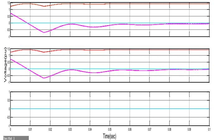
Figure 16: Simulation result of supply voltage and reference voltage and error signal in dq0
