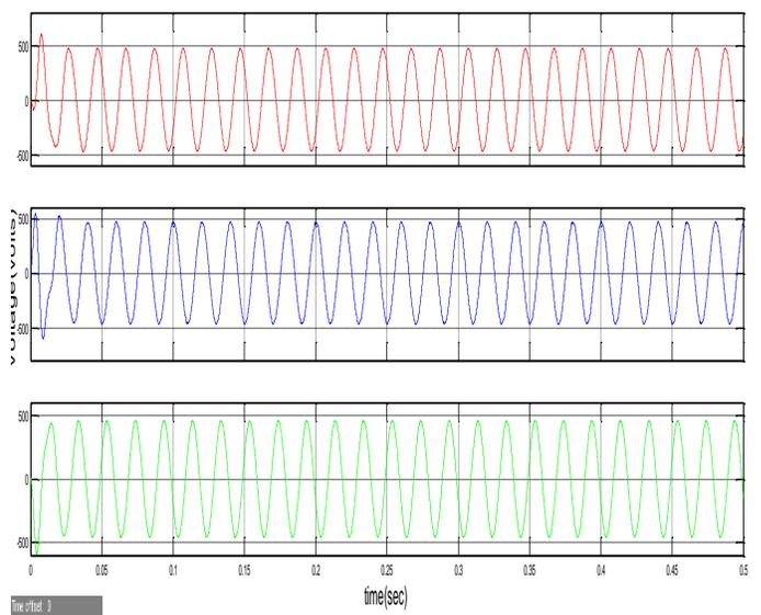
Figure 2.25: SPWM based inverter Voltage waveforms With Filter Circuit
