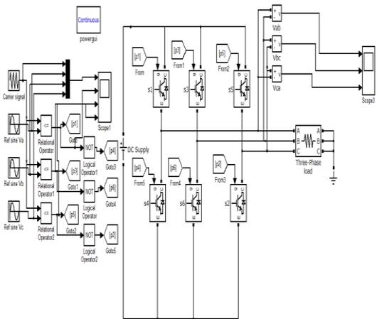
Figure 26: SPWM based inverter Without Filter Circuit
