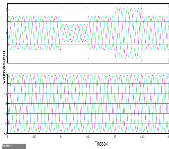
Figure 20: Simulation result of supply voltage and reference voltage in the event of sag and swell in all phases
