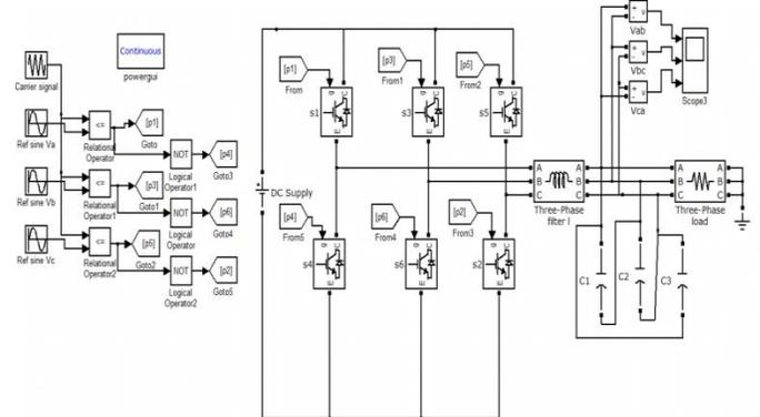
Figure 28: SPWM based inverter With Filter Circuit
