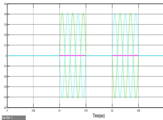
Figure 19: Simulation result of error signal in abc in the event of sag and swell in one phase
