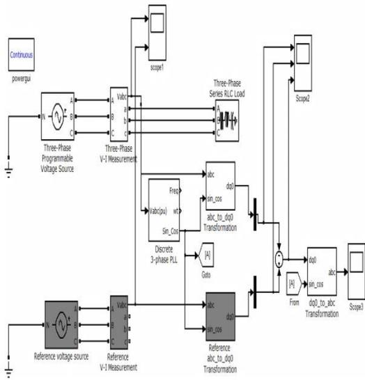
Figure 14 Simulation for system with error signal generated
