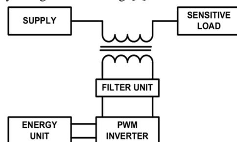
Figure 1 Typical applications of DVR and its output.
