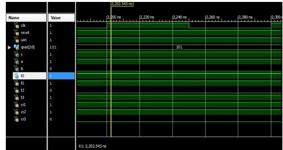
Figure 8. Simulation of the 5 mod serial residue generator
