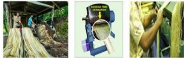
Fig. 2 Process Of Generation Of banana fiber.
