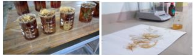
Fig.3 Submerging banana fibers in NaOH solution.
