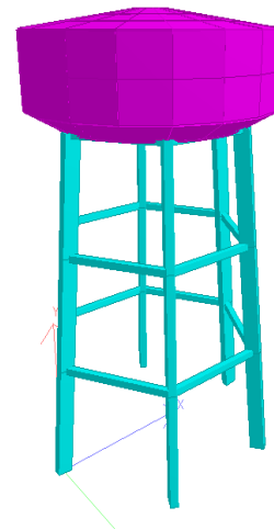
Figure 1: case 1 Intze type tank with inclined legs
