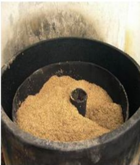
The ferro-cement furnace. Rice husk in the wire mesh cage.
