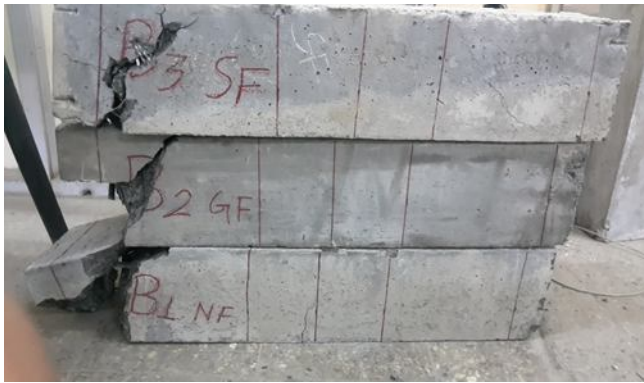
Fig. 7. The crack pattern and failure modes of the tested specimen
