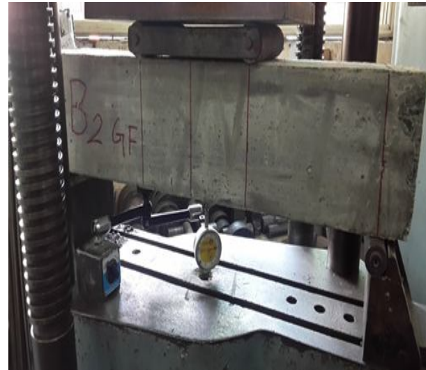
Fig. 6. Test set-up of the tested beam
