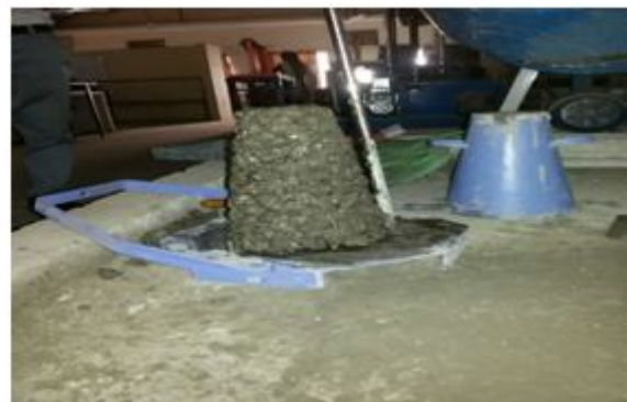
Fig no.1 Slump Cone Test
