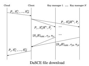
The file download process of DaSCE is depicted. The process starts with the client downloading the data from the cloud. To decrypt F, we need the K that is encrypted with Si. The Si is encrypted with (ei, ni), received from KM. The client establishes the session key with the KMs and during the process both the client and the KMs
