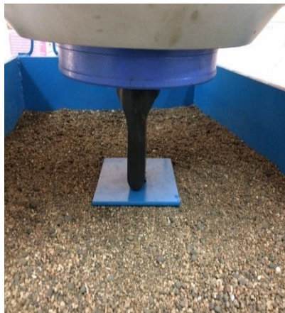
Fig 3. Photograph Showing loading on Piled –Raft Foundation
